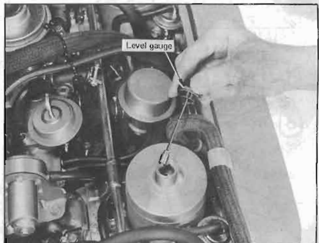
Fig. EF-35 Checking damper oil
